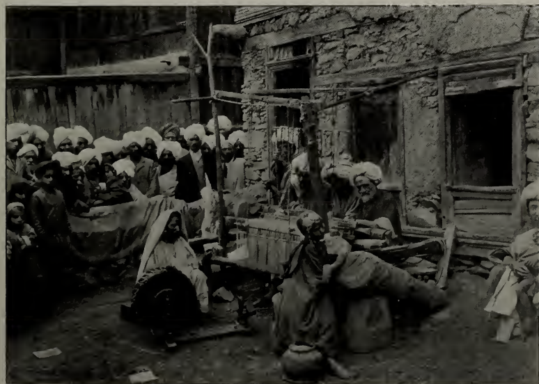
Men weaving and a woman spinning for Kashmir shawls, Kashmir State, India. An illustration to show primitive weaving and a "home-made" loom. Note also the keyed mortis construction at the corner of the wooden building in the rear, the framing of the house at the right and the decorative treatment of the spinning wheel.
